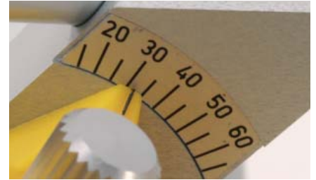
Condylar Housing inclination angle indicator
